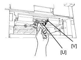
3. Clean the paper feed rollers [W] in the cassette with the soft damp cloth, while rotating them as shown in the diagram.
